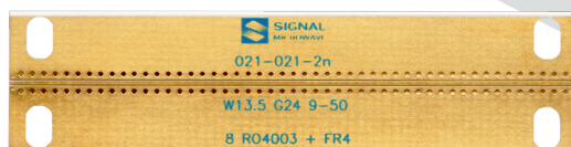
2" Grounded Coplanar Waveguide (GCPWG) on 8 mil RO4003 with FR-4 Backer
