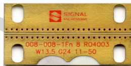
1" Grounded Coplanar Waveguide (GCPWG) on 8 mil RO4003 with FR-4 Backer
