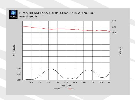
Typical test data through 27 GHz using FRM27-005NM-12 back-to-back connector pair with test pin.
