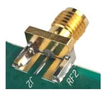
Typical Edge Mount Soldered Connector
