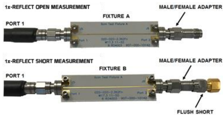
Figure 6: Setup example picture for measuring open and short for the 1x-reflect methodology.
