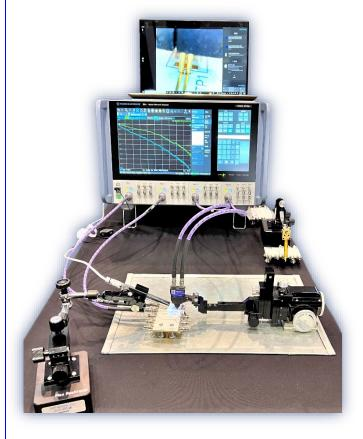
Scan the above QR code and share this technical application video with your design team in order to better understand how to accurately de-embed true differential probes thereby making more accurate time and frequency domain measurements.
