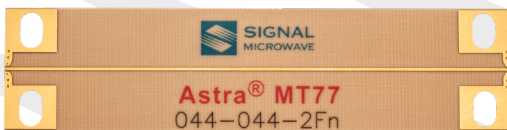
2" Microstrip on 5 mil ISOLA ASTRA MT77 with FR-4 Backer
