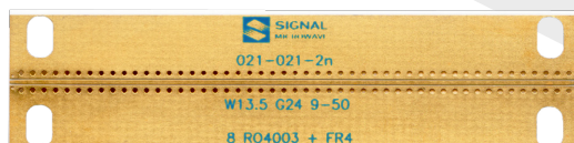
2" Grounded Coplanar Waveguide (GCPWG) on 8 mil RO4003 with FR-4 Backer
